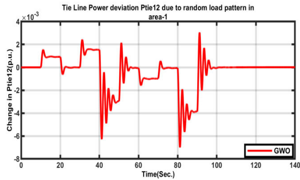
Fig.20 Tie Line Power Deviation in Area 1 & 2 due to Random Load Pattern
