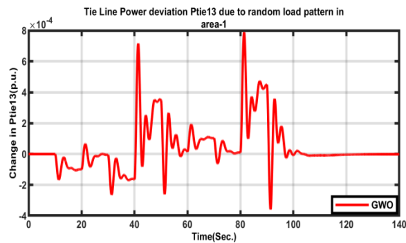
Fig.22 Tie Line Power Deviation in Area 1 & 3 due to Random Load Pattern
